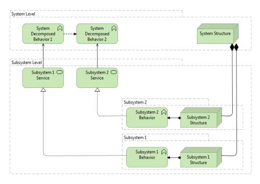
Figure 7. System decomposed behavior allocation
