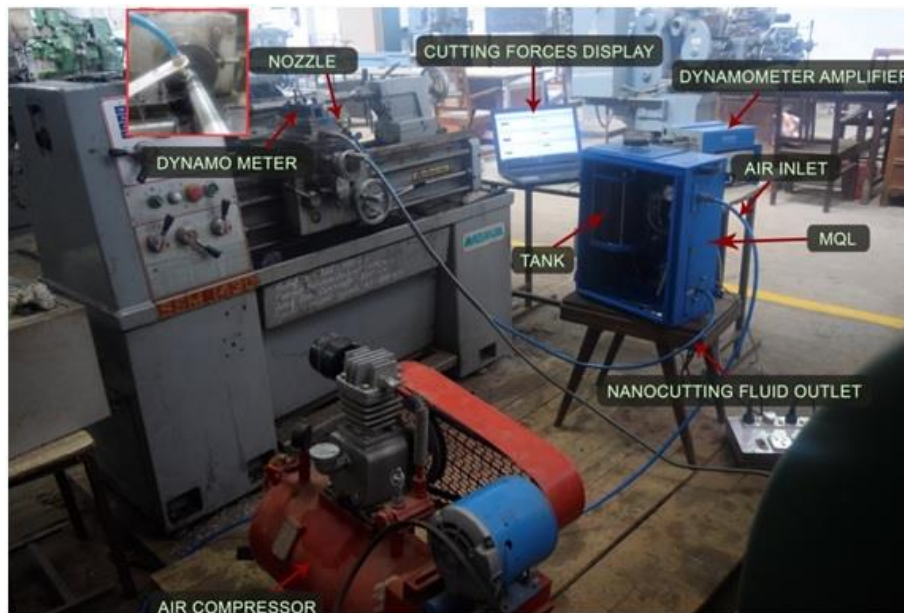
Figure 2. Machining experimental setup for turning under minimal quantity lubrication
