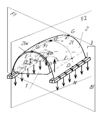
Figure 1. Scheme of the process of simple hanging over a tight punch of a shell of significant double curvature of a biconvex shape: 1 - punch; 2 - blank; 3 - press clamps
