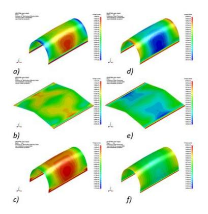
Figure 5. Distributions of experimental data 1 from the first kinematic scheme in the following stages: after the first skinning by an angle of 900 (a, d), after the part is bent through the angle 120 and its extension (b, e), at the end of the molding operation (c, f); a, b, c - distribution of effective deformations along the middle shell surface; d, e, f is the shell thickness distribution
