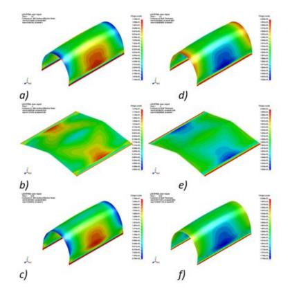
Figure 7. Distributions of the experimental data 14 from the third kinematic scheme in the following stages: after the first skinning by an angle of 900 (a, d), after the part is bent through the angle 120 and its stretching (b, e), at the end of the molding operation (c, f); a, b, c - distribution of effective deformations along the middle shell surface; d, e, f is the shell thickness distribution
