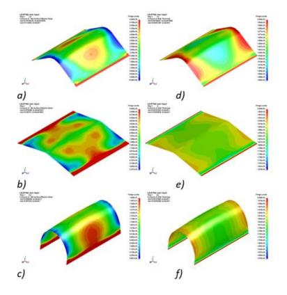
Figure 6. Distributions of experimental data 8 from the second kinematic scheme in the following stages: after the first skinning by an angle of 180 (a, d), after the workpiece has been bent by 120 and stretched (b, e), at the end of the molding operation (c, f); a, b, c - distribution of effective deformations along the middle shell surface; d, e, f is the shell thickness distribution
