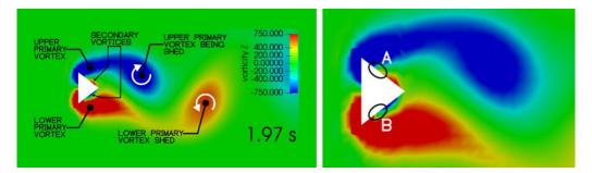
**Figure 6.** Nomenclature of primary and secondary vortices used in the study. The white arrows show the sense of rotation of the vortices. The region of inactivity identified by black ellipses in representative vorticity plot. The region marked by the letter A is located on the upper side of the triangular cylinder while the region marked by the letter B is located on the lower side of the triangular cylinder.
