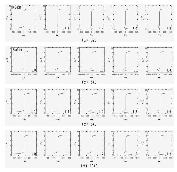
Figure 11. The z-component of vorticity at (a) Re = 520, (b) Re = 640, (c) Re = 840 and (d) Re = 1040.
