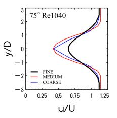
Figure 3. The figure shows a comparison between time-averaged and non-dimensionalised transverse *x*-component, "*u*" velocity profile at 8D downstream for coarse, medium and fine meshes. The velocity is non-dimensionalised by dividing *u* by free stream velocity,  $U = 2.5 \text{ ms}^{-1}$ . The *y*-axis distance, *y*, is non-dimensionalised by dividing it by base, D = 6 mm.
