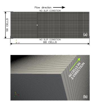
**Figure 4.** Details of three-dimensional mesh used in numerical simulations. (a) The figure shows the twodimensional view of the mesh, number of cells in both x and in y-direction and the faces where the no-slip condition is applied. The direction of flow is from left to right. (b) The figure shows the three-dimensional view of the mesh with the number of cells in z-direction.
