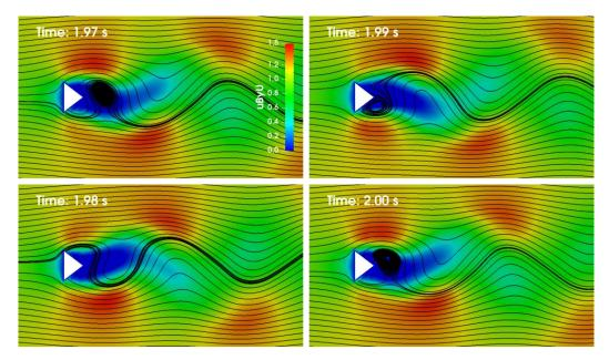
Figure 8. Streamlines superimposed on non-dimensionalised instantaneous x-velocities at Re = 1040. These velocities were non-dimensionalised by dividing with free stream velocity,  $U = 2.5ms^{-1}$ .
