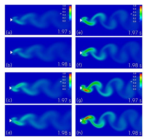
Figure 7. Instantaneous turbulent intensities at (a, b) Re = 520 (c, d) Re = 640 (e, f) Re = 840 (g, h) Re = 1040.
