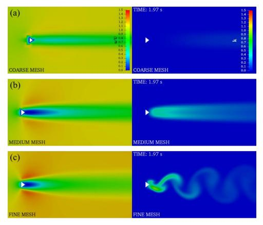
**Figure 2.** Comparison of non-dimensionalised time-averaged x-component of velocity, u, and instantaneous turbulent kinetic energy (TKE) at time, t=1.97 s at Re = 1040 ( $U = 2.5 ms^{-1}$ ) for 75° triangular cylinder in DOWN configuration for (a) coarse mesh, (b) medium mesh and (c) fine mesh. The velocity is non-dimensionalised by dividing u by free stream velocity,  $U = 2.5 ms^{-1}$ .
