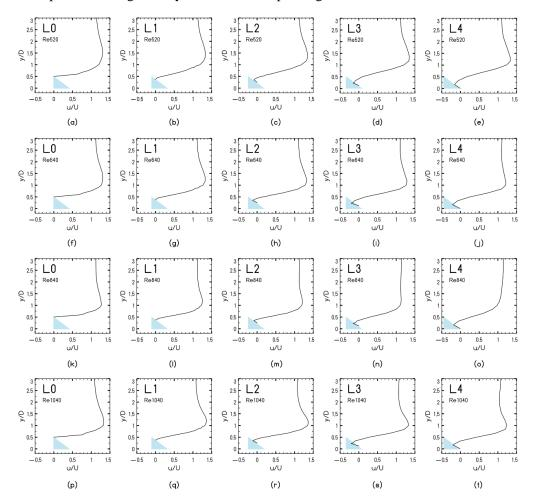
Figure 10. Instantaneous x-velocity component profile at equidistant locations on downstream cylinder surface at steady state at Re = 520, 640, 840 and 1040. The half blue triangle indicates the starting point of the line on the upper side of the triangular cylinder along which the data for velocity profile was extracted. The line was normal to the side of the triangular cylinder instead of being parallel to the base.
