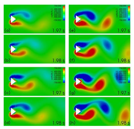
Figure 9. Instantaneous z-component of vorticity at (a, b) Re = 520 (c, d) Re = 640 (e, f) Re = 840 (g, h) Re = 1040.
