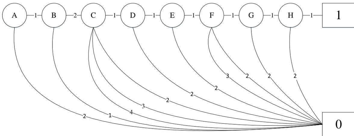
**Figure 4.** The MDD of the bogie system in state 2.
