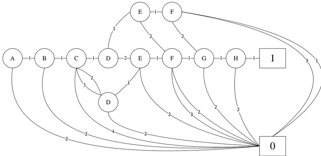
Figure 5. The MDD of the bogie system in state 3.
