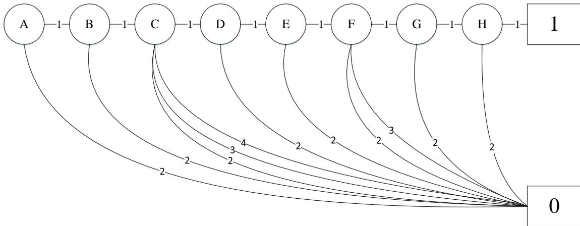
**Figure 3.** The MDD of the bogie system in state 1.
