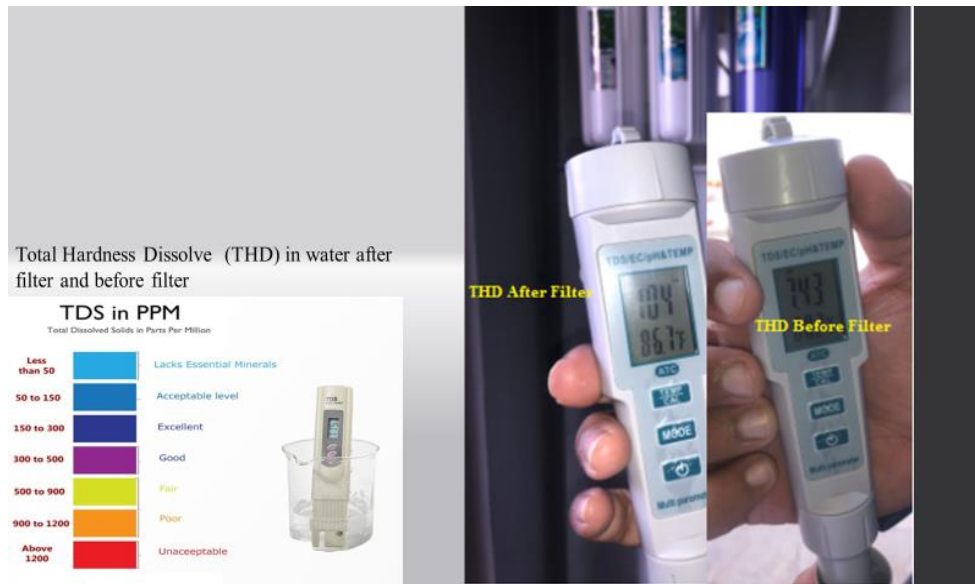
Figure 10. THD after filter and before filter.
